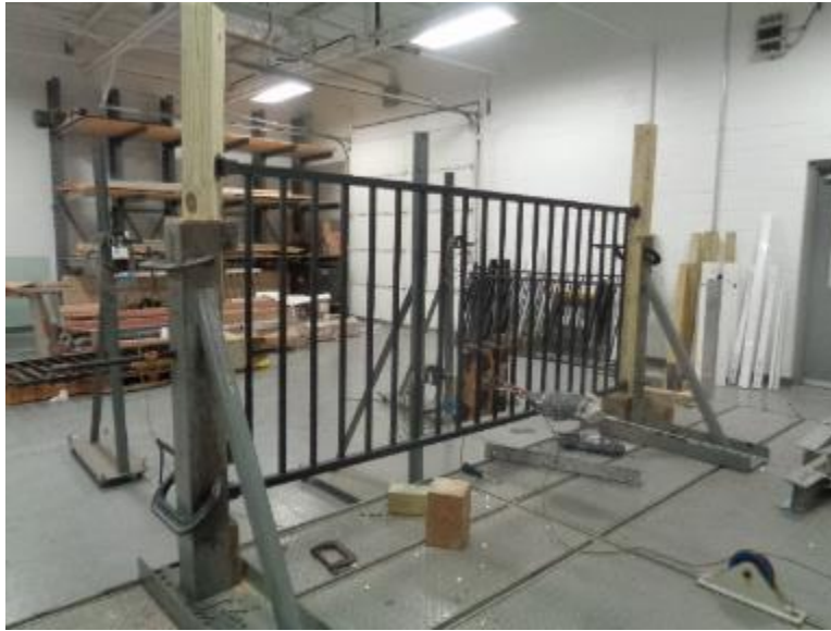
Photo No. 3 In-Fill Load Test at Bottom of Two Pickets
