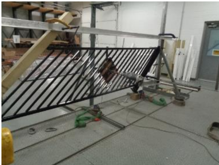
Photo No. 2 In-Fill Load Test at Center of Two Pickets
