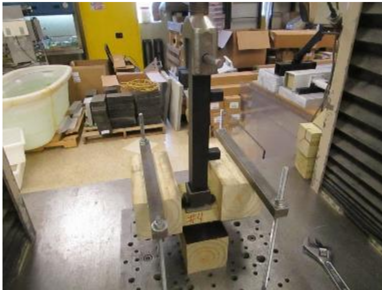
Photo No. 1 Assembly Fastener Test Setup
